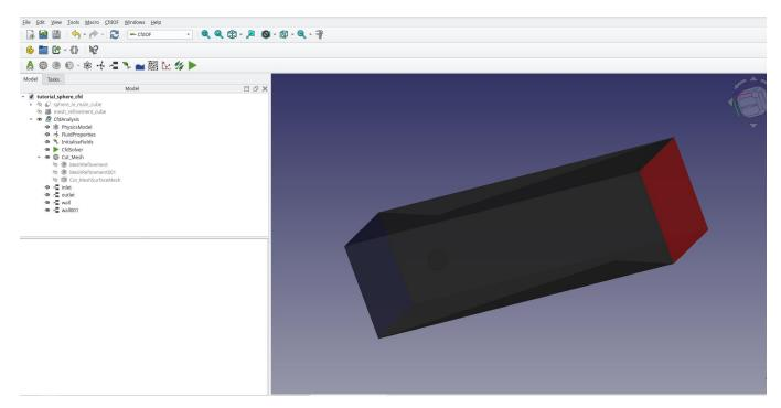
The next phase of this Cfd tutorial is to define the boundary conditions. In this particular case it is esentially defining which parts of the geometry form the walls, the inlets and outlets for our virtual wind tunnel. Additionally we'll also need to define the type of boundary our test sphere will have.
