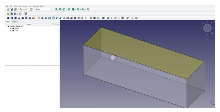
Starting in a new project we'll begin by modelling the target object for our computational fluid dynamic analysis. This of course could be anything, but let's start simple! We'll create a sphere and we'll insert it into a fluid domain, which is a fancy way of saying we'll put it inside a defined area filled with some kind of fluid. In our case a large volume we can think of as a virtual wind tunnel.
