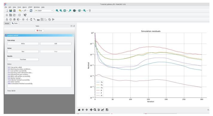
Excitingly we are now at the point where we run the CFD solver! First lets double click on the main mesh item in the analysis container, re write the mesh case and re run the mesh case to make everything up to date. If you omit this step when you start the actual solver it will probably prompt you to re-mesh at this point.
