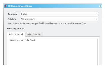
Next let's set the boundary conditions for the remaining 4 surface of our cube. Hold the control key whilst selecting the four faces of the cube in the preview window and then once again click the "Fluid boundary" tool icon. We can then simply set the boundary as "wall" and set the sub-type to "slip". Click OK to close the dialogue.
