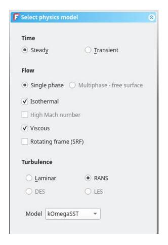
To set up the Physics Model double click on the Physics model item in the Cfd Analysis container. In the "Select physics model" dialogue that opens create the following settings. Set the "Time" to "Steady" and the "Flow" to "Single Phase" and check the "Isothermal" and the "Viscous" tickboxes.
